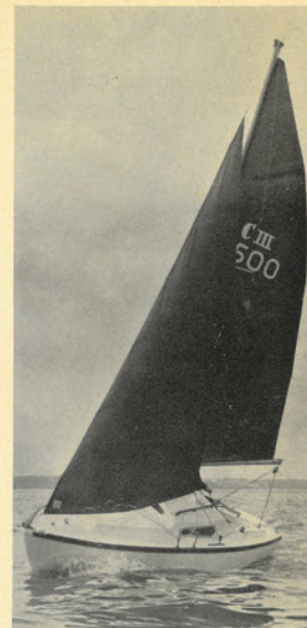
Above: in the Mark III version of the Caprice, the hard-chine plywood hull has been replaced by a round-bilged glass fibre one. The sails shown in this picture are the basic 75sq ft main, and 65sq ft working jib. A genoa and spinnaker are also available.
